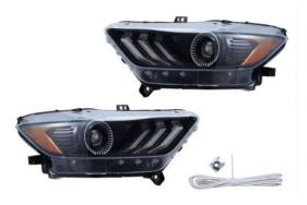
This headlight can be installed in both European and American models of Ford Mustang. If it is an US version of the car, please ignore the white and yellow lines behind the headlights and directly connect the black plug to the car.
