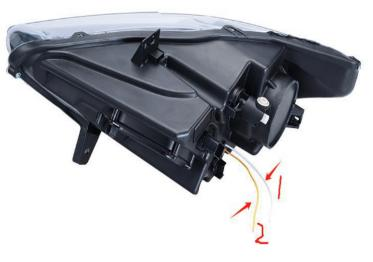
After connecting the two wires behind the headlights to the daytime running light function of the car, you can connect the plug behind the headlights to the car. This will enable the illumination of that area.
